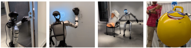
Fig. 7: Compliance enables contact-rich teleoperation like opening a door, wiping a whiteboard, dragging a chair while walking, and holding a rubber ball. C-GMT is robust to inevitable operator error when contact dynamics are unknown and imperceivable to the operator.
